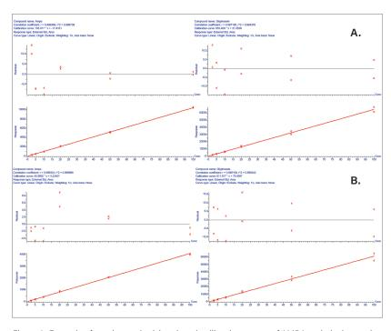
Figure 3. Example of matrix matched, bracketed calibration curves of AMPA and glyphosate in tomato (a) and cucumber (b) at 0.005 mg/kg-0.200 mg/kg.
