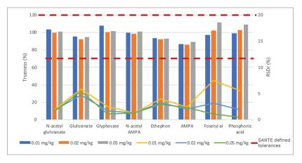
Figure 4. Percent trueness data at 0.010 mg/kg, 0.020 mg/kg, and 0.050 mg/kg spiking levels in tomato are plotted in the bar chart with the respective %RSDr plotted as lines on the secondary y-axis. The tolerances permitted by 11813/2017/SANTE are plotted in red for trueness (within 70 and 120%) and repeatability (< 20%).
