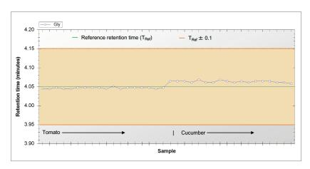
Figure 2. Retention time stability of glyphosate plotted in TrendPlot for the two commodities, each at n = 30, for samples spiked at various levels.
