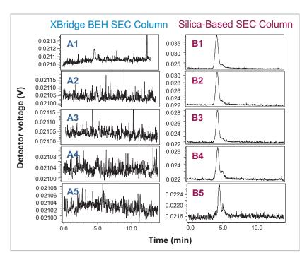
Figure 1. SEC-MALS baseline noise profiles for Channel 1 (43.6°) of a Wyatt miniDAWN TREOS MALS detector for the columns evaluated. Profiles A1 through A4 and B1 through B4 represent the first four blank injections on a new column after one hour of conditioning. Profiles A5 and B5 represent the third blank after a series of six samples.
