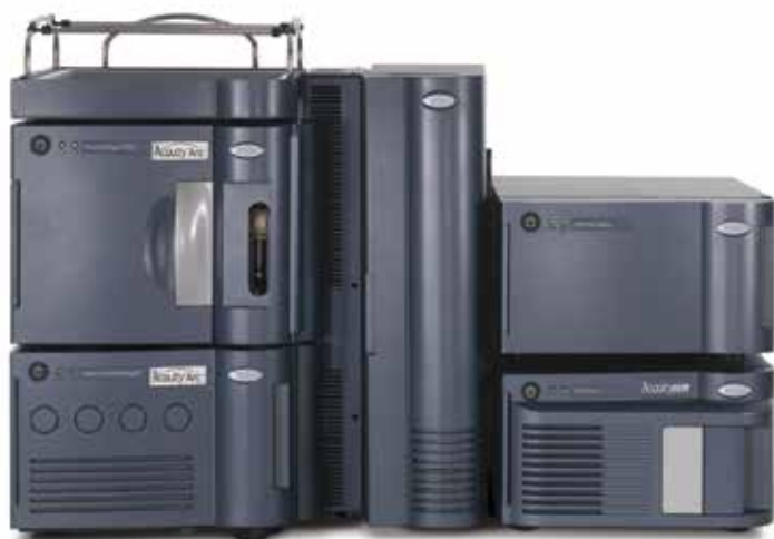
Figure 2. ACQUITY Arc System with the PDA and ACQUITY QDa detectors.
