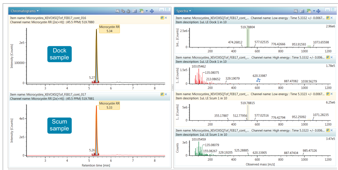
Figure 9. Extracted ion chromatogram and resulting spectra for microcystin-RR in the dock and scum samples.
