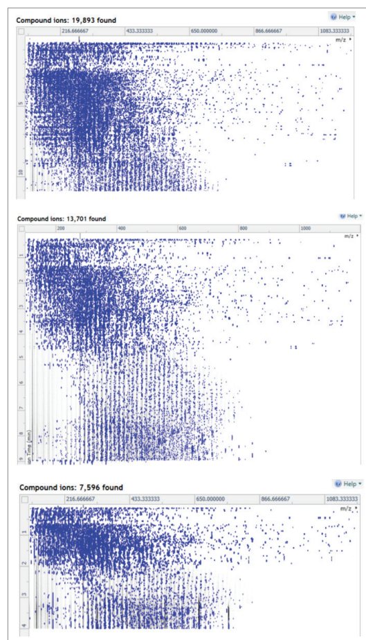
Figure 4. Peak density maps for the UPLC-IM-MS analysis of human urine. The top peak density map shows the results obtained using a 2.1 x 150 mm column and a gradient duration of 15 minutes with ion mobility separation enabled, the center peak density map shows the same sample analyzed using a 2.1 x 75 mm column and a gradient duration of 7.5 minutes with ion mobility separation enabled, the lower peak density map shows the same sample analyzed using a 2.1 x 30 mm column and a gradient duration of 3 minutes with ion mobility separation enabled.
