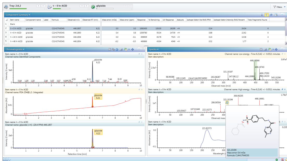
Figure 3. Low and high energy (MS E ) spectra and UV plot reported. The fragment ions are automatically assigned based on the structure (.mol file) of the API.
