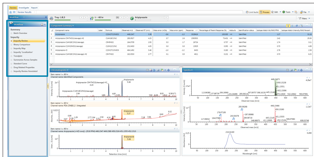
Figure 2. An example impurity identification workflow within UNIFI. The selected impurity review step shows an overview of the impurities identified in the component summary. The extracted ion chromatogram (XIC), UV chromatogram, and spectra are also shown as the component highlighted.
