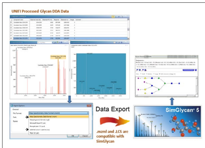
Figure 3. Workflow 2: Glycan DDA workflow in UNIFI Software. Collision-induced dissociation (CID) of glycans in data dependent acquisition (DDA) mode is processed and exported to SimGlycan.
