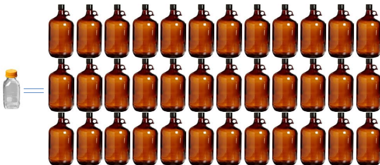
Figure 9. Comparison of relative solvent consumption of ionKey running at 7 \mu\text{L}/\text{min} flow rate vs. analytical scale chromatography running at 1 mL/min flow rate is displayed. The figure shows that consuming 1 L solvent on the ionKey/MS System running continuously at 7 \mu\text{L}/\text{min} for 99 days or 35,700 injections at 4 min run time, is equivalent to thirty six 1-gallon bottles using an analytical scale system.
