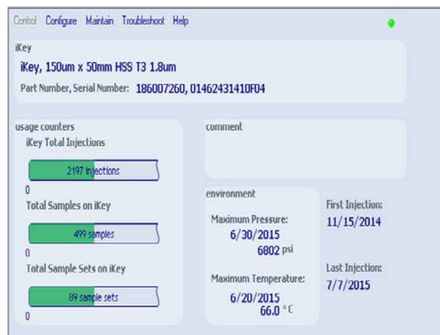
Figure 8. Screen capture of the HSS T3 iKey history, showing the number of injections (2197) and maximum operating pressure.
