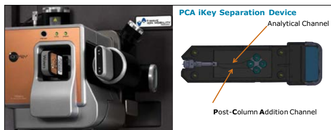
Figure 2. ionKey/MS source and PCA iKey Separation Device incorporating fluidic/electronic connections and ionization emitter.
