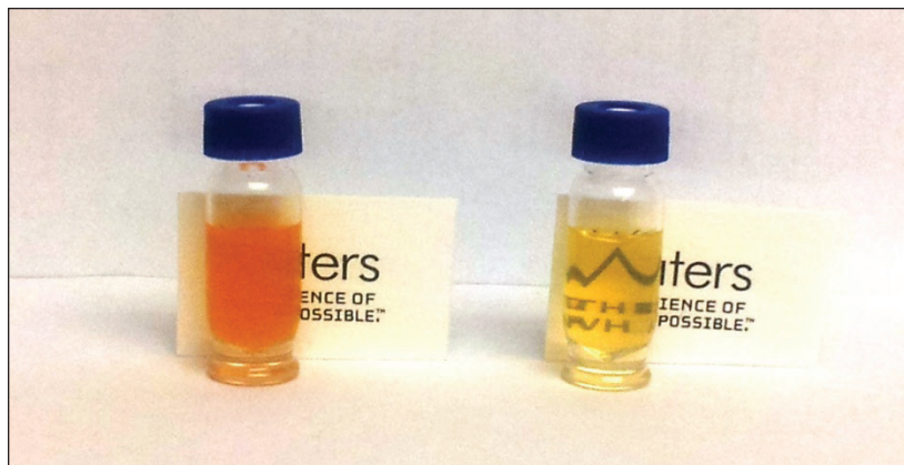
Figure 3. SPE cleanup for LC-MS. Vial on left shows a chili powder sample prepared with no dSPE cleanup; vial on right shows a sample prepared with dSPE cleanup.
