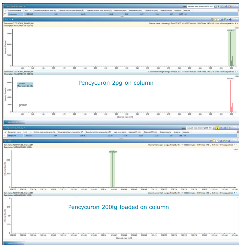
Figure 6. Accurate mass measurement (<1 ppm), precursor ions, ion mobility product ions, and collision cross sections (<1%) for confidence in identification, for pencycuron detected at 2 pg and 200 fg on column.
