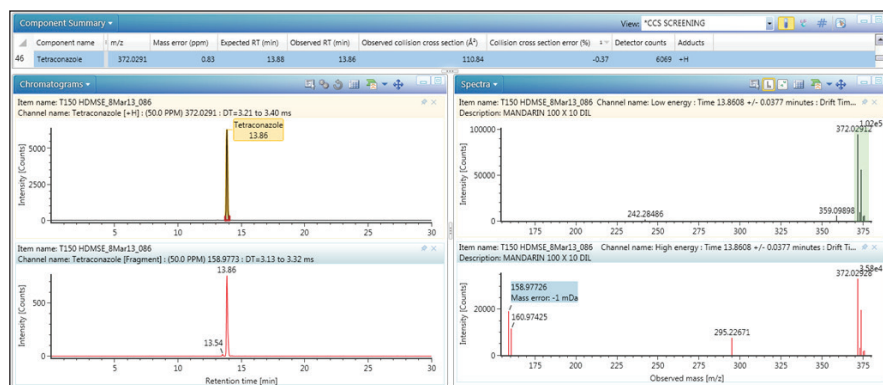
Figure 2. UNIFI Software Component Summary showing the response obtained for pesticide tetraconazole at 1 pg/ \mu L using the ionKey/MS System with ion mobility. Retention time and drift time aligned precursor ion and ion mobility product ion spectra are presented, with corresponding extracted mass chromatograms. Observed CCS values and CCS errors are presented along with retention time.
