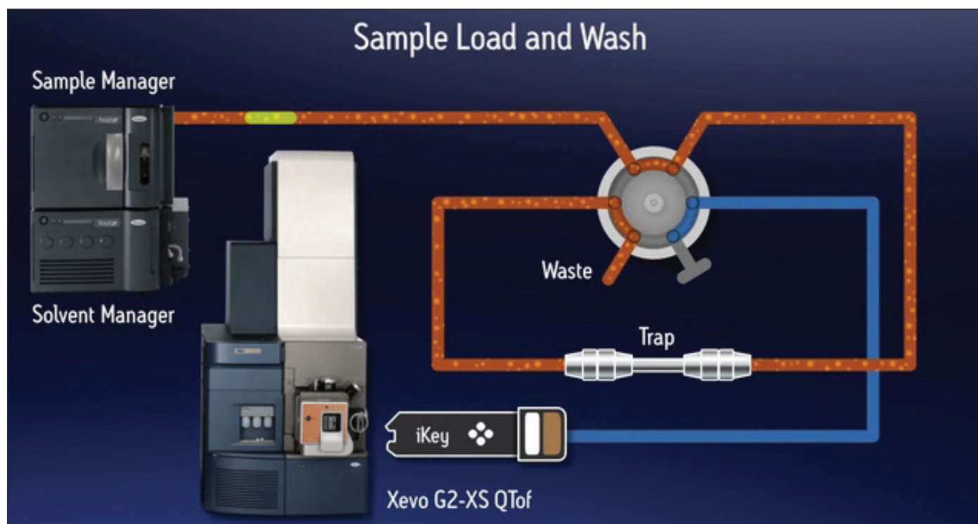
Figure 1. Schematic of the ionKey/MS System configured for single pump trapping.
