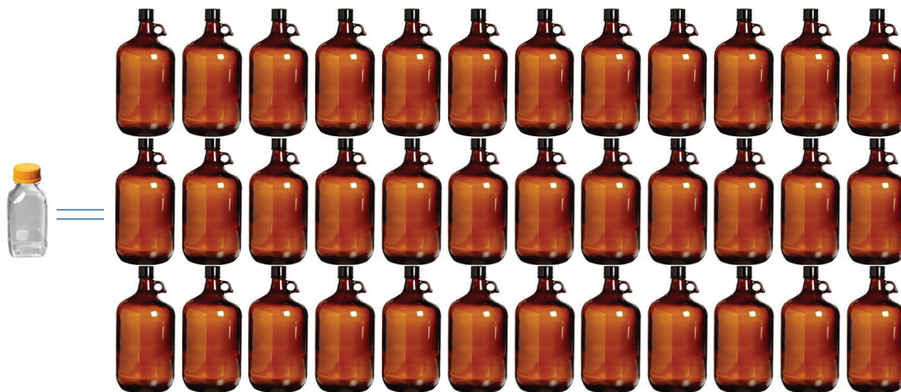
Figure 9. Comparison of relative solvent consumption of ionKey running at 7 \mu\text{L}/\text{min} flow rate vs. analytical scale chromatography running at 1 \text{ mL}/\text{min} flow rate is displayed. The figure shows that consuming 1 L of solvent on the ionKey/MS System running continuously at 7 \mu\text{L}/\text{min} for 99 days or 35,700 injections at 4 min run time, is equivalent to thirty six 1-gallon bottles using an analytical scale system.
