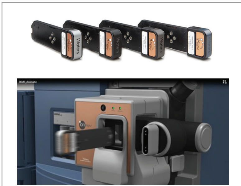
Figure 1. (top) Series of ionKey devices illustrating integrated chromatography-ESI. (bottom) Plug and play ionKey source illustrating insertion of iKey devices.
