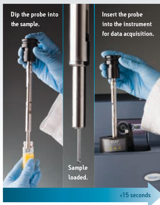
Figure 1. The sample is loaded directly onto the tip of a glass capillary. The sample is then directly inserted into the ionization source chamber. Bulk MS data are collected in seconds.
