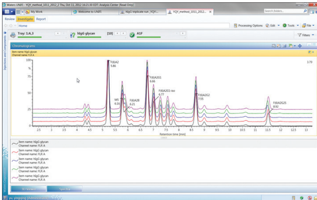
Figure 5. The Investigate panel of the experiment demonstrates glycan profile reproducibility for five HILIC UPLC FLR analyses of the glycan mixture.
