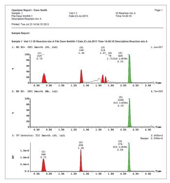
Typical MassLynx™-based Open Access report for a medicinal chemist using the ACQUITY UPLC I-Class PLUS System with ACQUITY QDa™ Mass Detector. The highlighted area shows how the ACQUITY QDa Mass Detector confirms that the required product (310 Da) has been successfully synthesized while the purity is determined from the ACQUITY UPLC PDA Detector.
