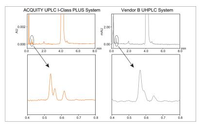
In this example, the impurity analysis of tetracaine was run under the same conditions on the ACQUITY UPLC I-Class PLUS System (system band spread of 4  $\mu$ L) and a UHPLC system (system band spread of 20  $\mu$ L). Although the UHPLC system was optimized for lowest possible dispersion and system volume, the impact of system dispersion is clearly evident. Significantly better resolution was achieved with the ACQUITY UPLC I-Class PLUS System.
