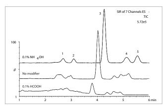
Figure 1. UPLC/MS analysis of carbohydrates in 75/25 ACN/H<sub>2</sub>O containing formic acid, no modifier, and ammonium hydroxide. The flow rate is 0.13 mL/min, the column temperature is 35 °C, and the Injection volume is 0.7  $\mu$ L. The concentration of each analyte is 10  $\mu$ g/mL in 50/50 ACN/H<sub>2</sub>O. The column dimensions are 2.1 x 50 mm, 1.7  $\mu$ m. Peaks: (1) fructose, (2) glucose, (3) sucrose, (4) maltose, and (5) lactose.
