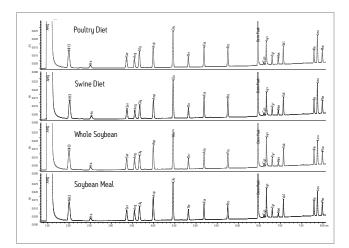
Animal feed hydrolysates, 6 ng on column, using the UPLC Amino Acid Analysis Solution.
