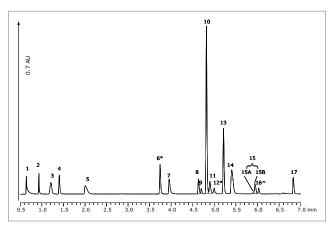
Chromatogram showing solvent standards with concentrations of approximately 5 ng/ $\mu$ L. All extracted at 270 nm, except compounds 6, 12, and 16. \* Extracted at 205 nm. Extracted at 630 nm.
