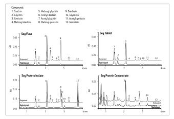
Figure 3. UPLC analysis of extracted (top chromatograms) and hydrolyzed (bottom chromatograms) candidate Standard Reference Materials (cSRMs).
