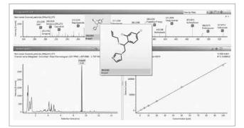
UNIFI component plot (upper data panel) shows the pesticide residues identified in a test sample and the calibration series for imazalil (1 to 100 ppb) and correlation coefficient R2=0.999.
