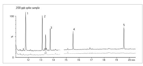
Figure 1. GC/MS chromatograms of unspiked ground beef samples (blue trace), and ground beef samples spiked with 200 ppb organophosphorus pesticides (black trace).
