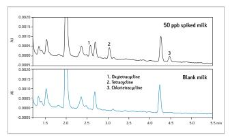
A typical HPLC/UV chromatogram (355 nm extracted wavelength, **XP** Column) obtained from analysis of a sample spiked with 50 ppb (ng/g) of three tetracyclines.
