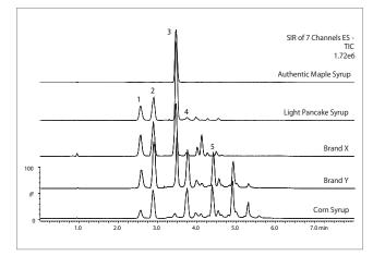
Figure 5. UPLC/MS analysis of carbohydrates in different maple syrups. Conditions are identical to Figure 3. Peaks: (1) fructose, (2) glucose, (3) sucrose, (4) maltose, and (5) maltotriose.
