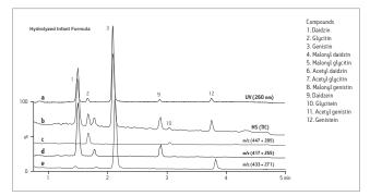
Figure 5. UPLC analysis of isoflavones in a commercially-available, soybased infant formula (after hydrolysis); a) UV [260 nm], b) MS - Total Ion Chromatogram [TIC], c) extracted ion chromatogram for m/z 447 + 285 [glycitin and glycitein], d) extracted ion chromatogram for m/z 417 + 255 [daidzin and daidzein], and e) extracted ion chromatogram for m/z 433 + 271 [genistin and genistein].
