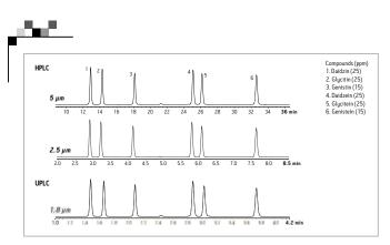
Figure 2. HPLC and UPLC separations (UV) of soy isoflavone standards on cyano columns: XSelect<sup>®</sup> HSS Cyano, 5  $\mu$ m, 4.6 x 150 mm (top); XSelect HSS Cyano **XP**, 2.5  $\mu$ m, 4.6 x 75 mm (middle); and ACQUITY UPLC HSS Cyano, 1.8  $\mu$ m, 2.1 x 50 mm (bottom). The gradient profiles, flow rates, and Injection volumes were scaled for each method using the ACQUITY UPLC Columns Calculator. The flow rates were 1.0 mL/min, 2.0 mL/min, and 0.58 mL/min, respectively.
