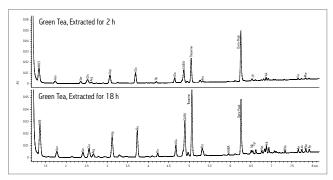
Two separate aliquots of a single type of green tea using the UPLC Amino Acid Analysis Solution. Each aliquot was extracted for 2 or 18 hours. Theanine (5.1 minutes) was confirmed by MS detection. All amino acid levels increase with duration of extraction.
