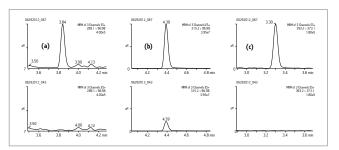
Figure 2. UPLC/MS/MS chromatograms of steroids obtained from milk samples; the top trace is the low level spiked sample, the bottom trace is a milk blank. (a) testosterone (b) progesterone (c) dexamethasone.
