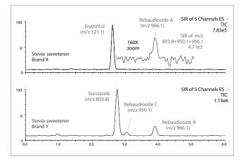
Figure 6. UPLC/MS analysis of two commercially-available stevia-related sweeteners. Isocratic mobile phase of 77.5/22.5 ACN/H<sub>2</sub>O with 0.1% NH<sub>4</sub>OH. The flow rate is 0.2 mL/min, the column temperature is 35 °C, and the Injection volume is 1.3  $\mu$ L. The concentration of the Brand Y product is 50  $\mu$ g/mL each in 50/50 ACN/H<sub>2</sub>O. The Brand X product is prepared at 10  $\mu$ g/mL in 50/50 ACN/H<sub>2</sub>O. The column dimensions are 2.1 x 100 mm, 1.7  $\mu$ m.
