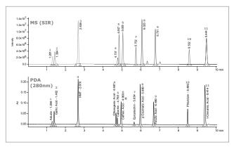
Simultaneous acquisition of PDA and MS (SIR) data for a 10 ppm standard mix in a single analysis.
