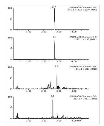
Figure 6. MRM chromatograms from an extract of a 1 ppb spike in baby food.
