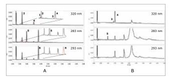
Typical chromatograms of vitamins A and E by UPC<sup>2</sup> with PDA detection. (A) standards; (B) Infant formula sample. Peaks: 1 cis-retinyl acetate, 2 all trans-retinyl acetate, 3 cis-retinyl palmitate, 4 all trans-retinyl palmitate, 5 alpha-tocopheryl acetate, and 6 alpha-tocopherol.
