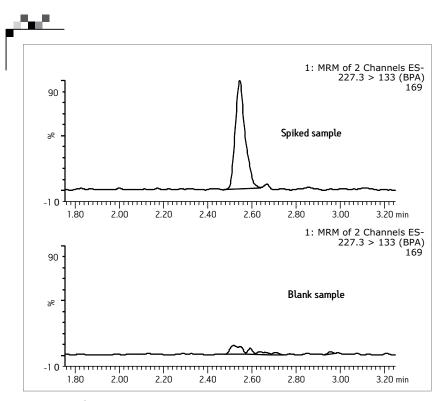
Figure 1. UPLC<sup>®</sup>/MS/MS chromatograms obtained from infant formula samples. The top trace is a 2 ng/g spiked sample, and the bottom trace is an infant formula blank.
