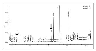
Figure 4: Different free amino acid profile of two commercially-produced pale ales. Arrows indicate significant differences between brands. Table 1: Lot-to-lot variability for one brand of pale ale. The values (expressed as pmoles/µL sample) include triplicate injections of two derivatizations.
