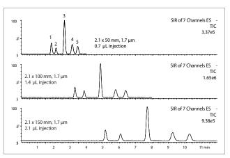
Figure 2. UPLC/MS analysis of carbohydrates using acetone as the organic solvent. The isocratic mobile phase was 77/23 acetone/H<sub>2</sub>O with 0.05% NH<sub>4</sub>OH. The flow rate is 0.13 mL/min and the column temperature is 85 °C. The column dimensions and Injection volumes are shown on the figure. The sample and peak elution order is identical to Figure 1.
