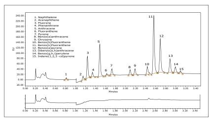
Figure 1. LC/FLR chromatogram obtained from a shrimp sample spiked with 20 ppb PAH compounds. The bottom chromatogram is an unspiked shrimp blank.
