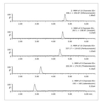
UPLC/MS/MS chromatogram obtained from DisQuE Pouch extract of orange juice spiked at 10 ng/g (ppb) of each fungicide (except 1 ppb carbendazim).
