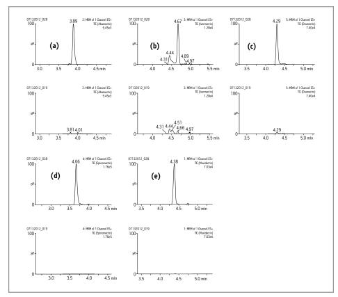
Figure 2. LC/MS/MS chromatograms of avermectins obtained from whole milk samples; the top trace is the low level spiked sample, the bottom trace is a whole milk blank. (a) abamectin (b) ivermectin (c) doramectin (d) eprinomectin (e) moxidectin.
