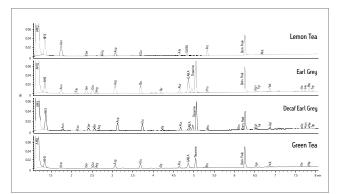
Extracted teas using the UPLC Amino Acid Analysis Solution. Theanine was confirmed by MS detection. Amino acids levels vary with type of tea.
