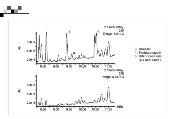
LC/UV (220 nm) chromatograms obtained on an XP Column from a DisQuE Pouch extract of orange juice spiked at 100 ng/g (ppb) after Oasis MCX cleanup.
