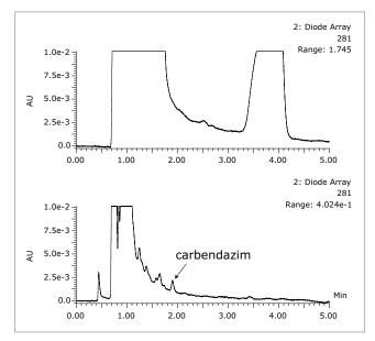
LC/UV chromatograms (281 nm) obtained from a DisQuE Pouch extract of an orange juice sample with incurred carbendazim. The top chromatogram was obtained with no SPE cleanup, while the bottom chromatogram was obtained after cleanup with the Oasis MCX Cartridge.
