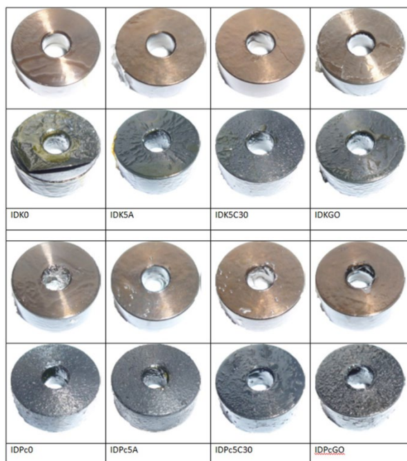
Fig. 1. Samples of depleted uranium coated with polymer protective layer before and after corrosion test (100h, 117 °C).
