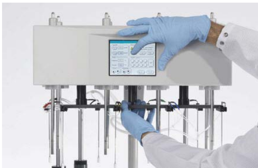
Figure 5-2. Installation of the Manifold
