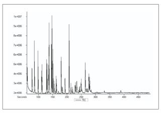
Figure 1. Total Ion Chromatogram (TIC) of silylated standard mixture at 2  $\mu$ g/mL.
