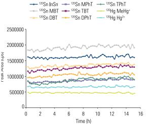
Figure 3: Stability of trace elemental species over a period of 15 h of repeat injections.
