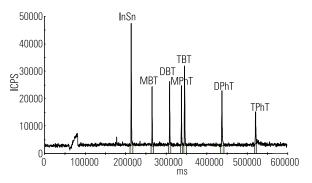
Figure 4b: Chromatographic data for a 0.1 ng/ml standard of various Sn species displayed in the XSERIES 2 PlasmaLab software.
