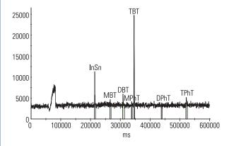
Figure 4a: Chromatographic data for a blank injection displayed in the XSERIES 2 PlasmaLab software.
