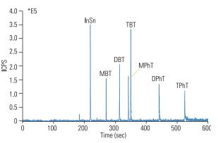
Figure 6b: Chromatographic data for a 0.1 ng/mL injection on the ELEMENT 2 displayed in Xcalibur Qual Browser.
