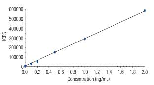
Figure 5: Calibration curve generated in PlasmaLab for MBT.
