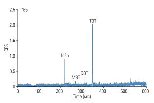
Figure 6a: Chromatographic data for a blank injection on the ELEMENT 2 displayed in Xcalibur™ Qual Browser.
