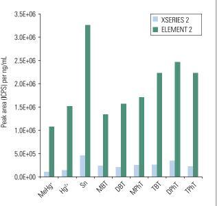
Figure 9a: Sensitivity per ng/mL for the XSERIES 2 and ELEMENT 2.
