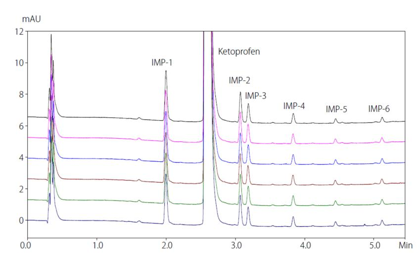
Fig. 3 Chromatograms of the Ketoprofen Standard Samples
