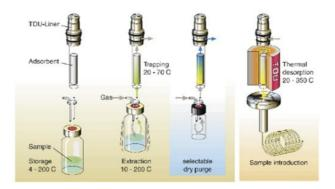
Figure 2 – Schematic view of the DHS Process
