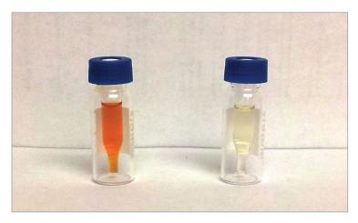
Figure 3. SPE cleanup for GC-MS; vial on left shows a chili powder sample with no cleanup, vial on right shows a sample after cleanup using carbon/PSA cartridge.
