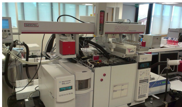
Figure 1: Gerstel Single Head MPS with GC/MS Single Quadrupole
