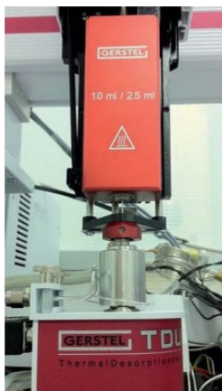
Figure 2: Detail photograph of a HIT injection
