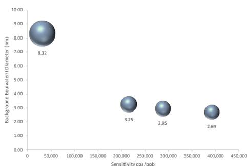
The relationship between calculated background equivalent diameter and instrument sensitivity (cps/ppb) for the analyte element.
