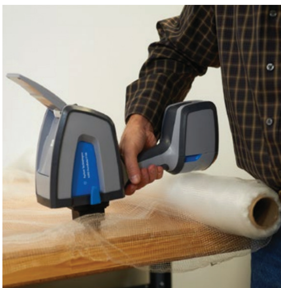
Figure 1. Agilent's 4300 Portable FTIR offers easy identification of polymers
