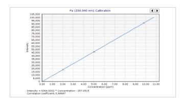
Figure 1. Calibration curve for Fe 259.940 nm.
