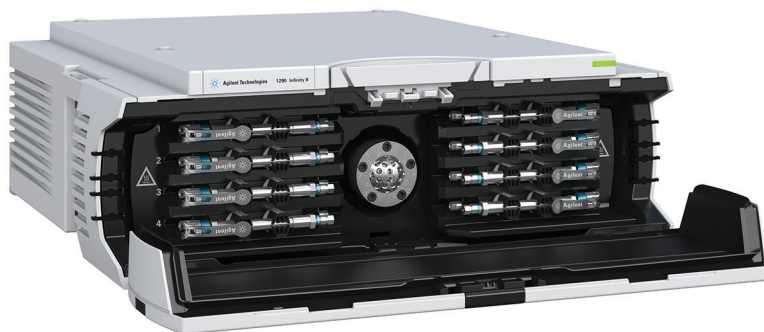
Figure 1. The Agilent 1290 Infinity II Multicolumn Thermostat holds up to eight columns, each with a distinct heat exchanger, in two independent temperature zones.
