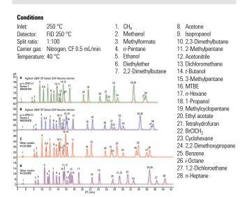
Multi-component mixture separated on two Agilent J&W CP-Select 624 Hexane columns from different series (A and B, p/n CP9111) and two columns from another vendor (C and D).
