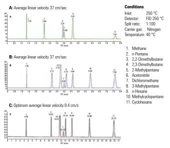
Separation of hexane isomers, acetonitrile, and dichloromethane on an Agilent J&W CP-Select 624 Hexane, 30 m x 0.32 mm, 1.8 µm GC column (p/n CP9111).
