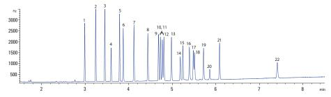
In just 7.5 minutes, we achieved complete analysis and confirmation of CLP pesticides. What's more, the excellent selectivity of this column pair allows you to meet the demands of up to 9 EPA methods on a single instrument.
