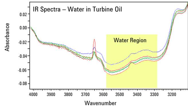
**Figure 1.** The overlaid IR spectra of turbine oil with the water absorbance region expanded, water values from bottom to top are 30 ppm (red), 80 ppm (dark green), 217 ppm (light green), 533 ppm (red), and 1460 ppm (blue)
