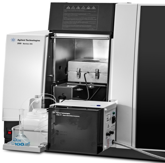
Figure 2. The ETC 60 electrothermal temperature controller (metal box in burner compartment) is an optional accessory for use with the VGA 77.
