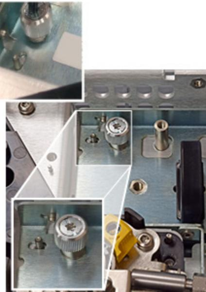
**8** Using the black handle, slide the detector module forward until it stops (about 3 mm)
