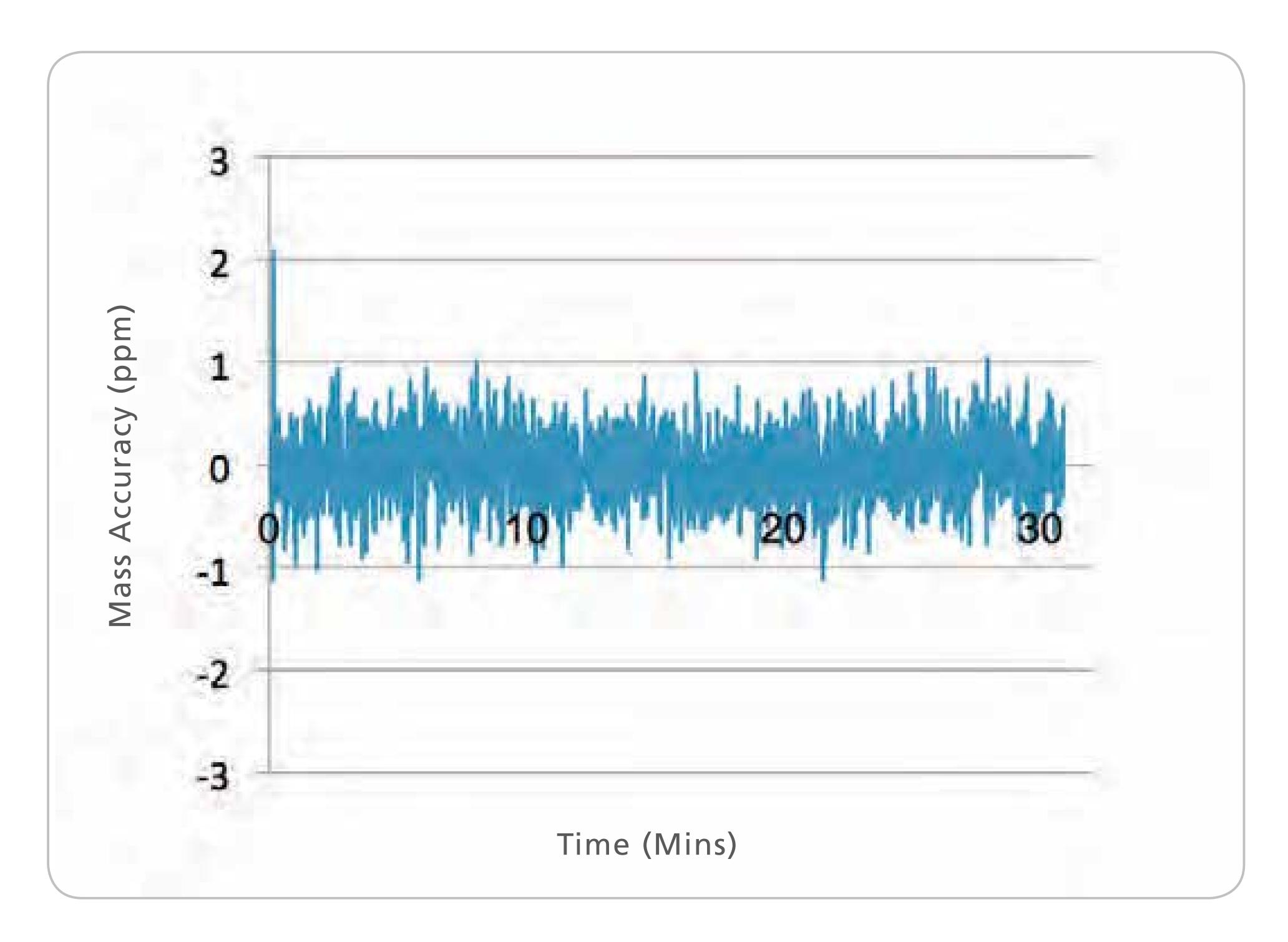
EasyMass(TM) accuracy delivers high mass accuracy MS and MS/MS data with ease. With external calibration, the mass accuracy holds rock-steady at <1ppm over 30 minutes, and RMS=1.69 over 100 hours.
