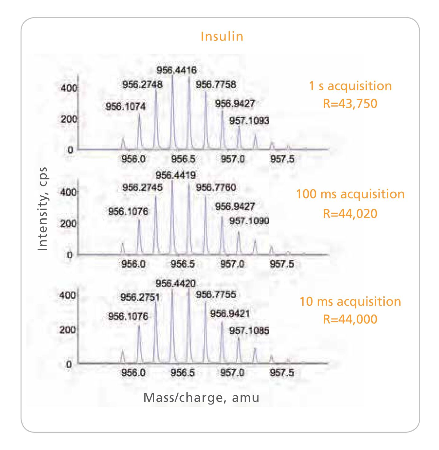
Resolution of insulin (6+) is maintained at >43,000 with data accumulation times of 1 second, 100 milliseconds, and 10 milliseconds.
