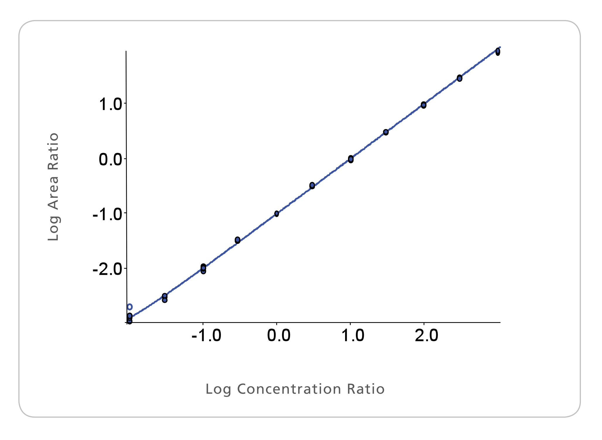
The system also provides up to 4 orders of magnitude linear dynamic range high-resolution, high-sensitivity data with acquisition speed up to 100 spectra/sec makes the TripleTOF 5600 system a perfect compliment to ultra-fast chromatography. The system also provides 4-5 orders of magnitude of linearity to ensure accurate quantitation in MS and MS/MS modes.
