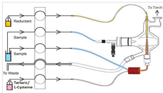
Figure 1. MSIS setup for dual mode, with an in-line pre-reduction mixing solution.
