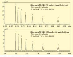
Chromatographic conditions: Column: described above; Mobile phase: water/acetonitrile (3/7, v/V); Flow rate: described above; Temperature: 40 °C; Detection: absorbance at 245 nm; Sample volume: 4 µL (XR-ODS), 10 µL (VP-ODS) Peaks: 1: Acetophenone, 2: Propiophenone, 3: Butyrophenone, 4: Valerophenone, 5: Hexanophenone, 6: Heptanophenone, 7: Octanophenone Top: Shim-pack XR-ODS / Bottom: Shim-pack VP-ODS
