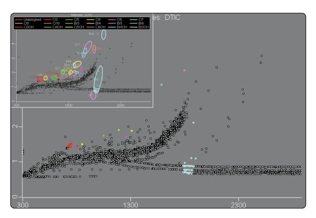
A plot showing only peak markers for an analysis of fish plasma by GCxGC-TOFMS. White Peak Markers are for unclassified peaks and colored Peak Markers correspond to peaks that have been classified. The inset shows the corresponding Legend and Classification Regions. This plot can be produced by selecting "No Contour" on the "Type" tab in "Properties".
