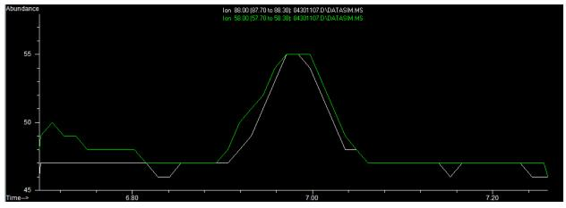
Figure 1: Extracted Ion Chromatogram (EIC) of a 10 ppb 1,4-Dioxane Standard
