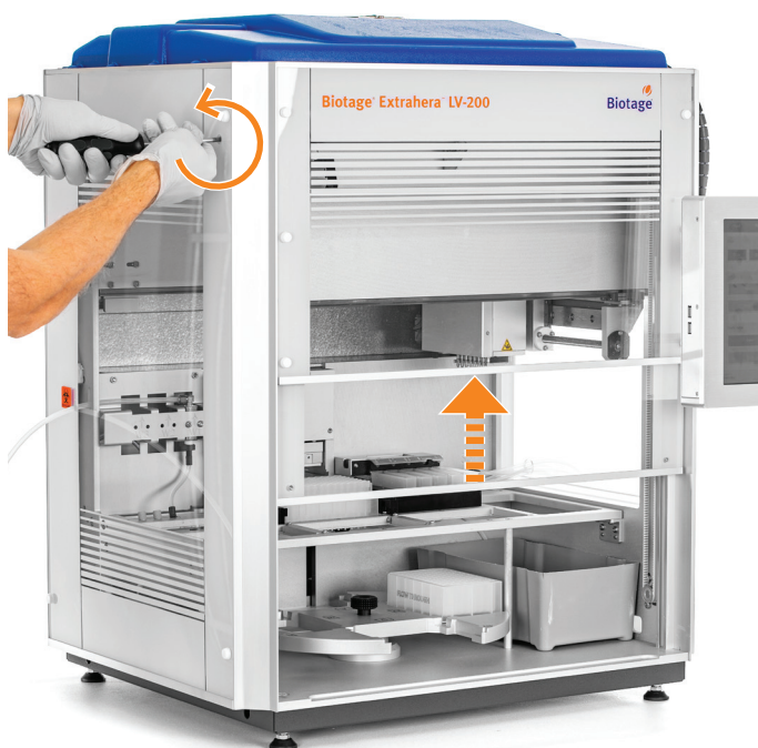
Figure 15. Open the door manually by turning the screw counterclockwise.
