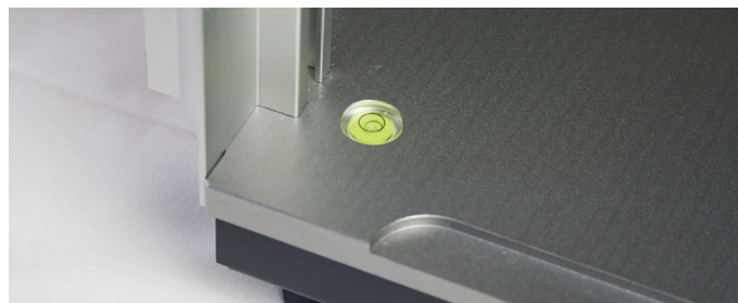
Figure 8. The built-in spirit level in the bottom of the system, in the front left corner.
