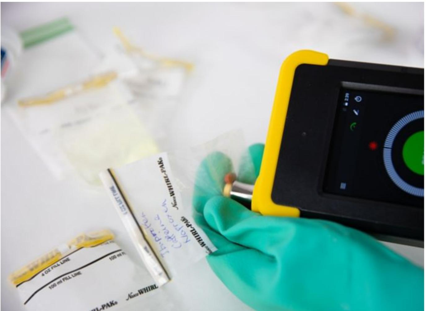
The TacticID Mobile® handheld Raman system from B&W Tek employs a 1064 nm laser, and can be used to quickly identify illicit substances in the field with the push of a button. The TacticID Mobile is able to suppress fluorescence and can identify more substances than traditional 785-nm Raman systems.
