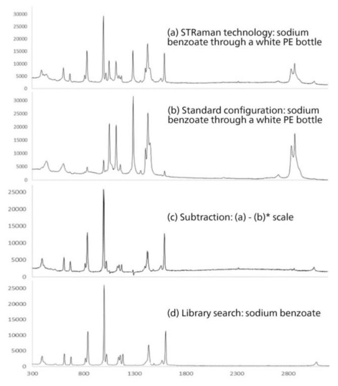
**Figure 1.** STRam identification of sodium benzoate through a white polyethylene bottle: (a) Spectrum measured through the bottle using the STRaman technology; (b) spectrum measured with a standard Raman configuration; (c) the result of scaled subtraction of (b) from (a); and (d) pure spectrum of sodium benzoate.
