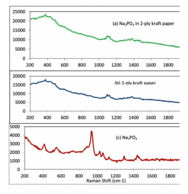
**Figure 3.** STRam-1064 identification of trisodium phosphate in bilayer bag of white and brown kraft paper layers (a) Spectrum measured through the bilayer bag using the STRaman technology; (b) spectrum of the bilayer bag measured with standard Raman configuration; (c) pure spectrum of trisodium phosphate.
