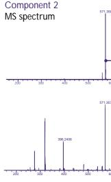
Component 2. In the MS spectrum the mass difference between m/z733.4494 and m/z571.3589 is 162.0905 (u). This mass difference is 14.0144 (u) and corresponds to CH<sub>2</sub> (14.0156 (u)). As the m/z396.2406 ion is present (Area A) and the ion at m/z571.3575 is also present (relating to the loss of Area A and a CH<sub>2</sub>group) the data is consistent with the loss of a methyl group in Area A.
