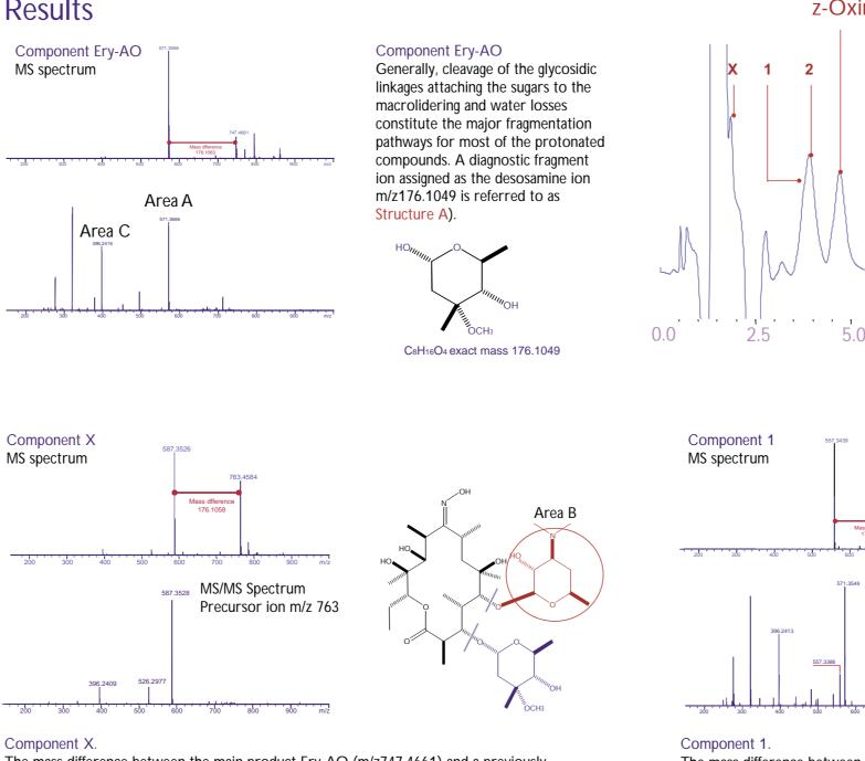
The mass difference between the main product Ery-AO (m/z747.4661) and a previously unknown Impurity labeled 'X' (m/z763.4584) is 15.9923 (u). This mass difference is equal to Oxygen, O (15.9949(u)) and provides strong evidence that this impurity has the structure with a single Oxygen atom in 'Area B' of the molecule
