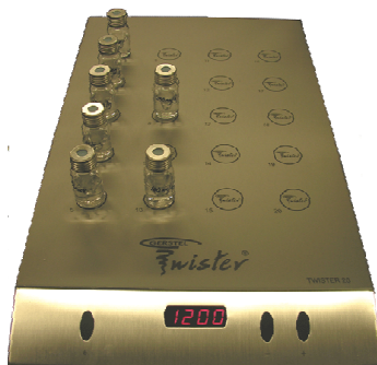
Figure 3: Photograph of a typical twister extraction.
