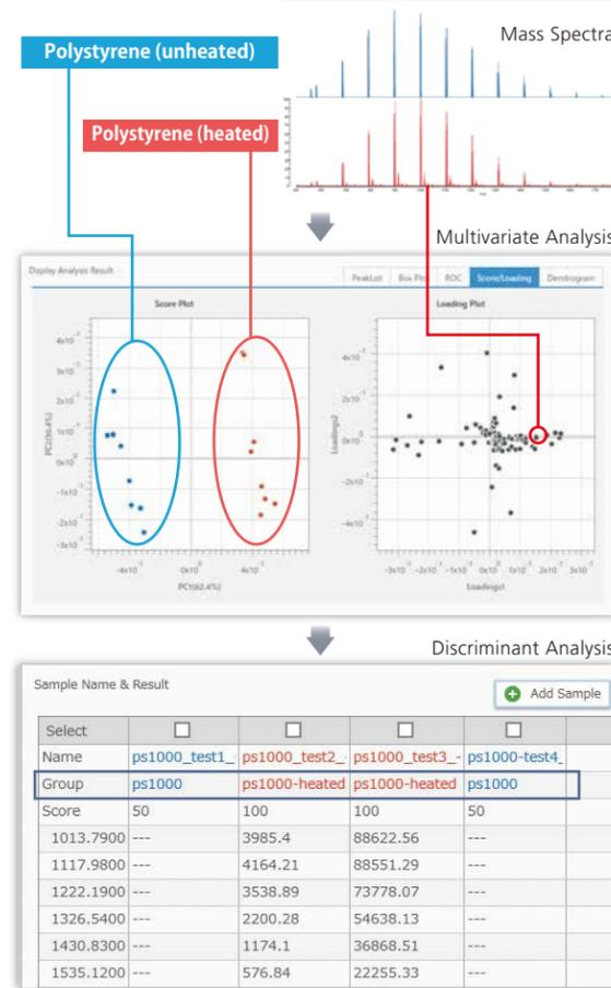
Polystyrene (heated and unheated) polymers were separated into two groups (heated or unheated) by multivariate analysis (PLS-DA) of the MALDI mass spectrum (Score Plot). A Loading Plot can be used to confirm which peaks (marker peaks) affect the differences between the two groups.
