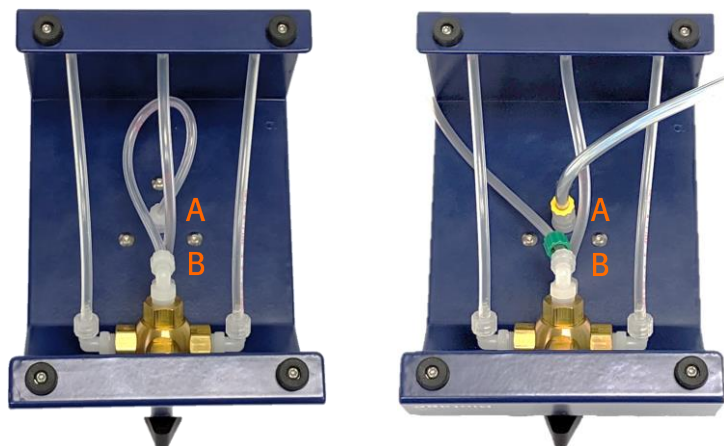
Figure 1. Replace the existing line connected to the sample port (A) and feed port (B) with the feed line and waste line of the One-Pass Kit.
