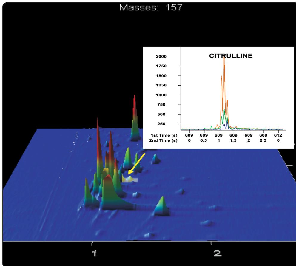
**GCxGC-TOFMS analysis of blood plasma sample with clear separation and identification of trace concentration of Citrulline an  $\alpha$ -amino acid.**
