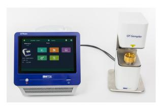
The QTRam®, powered by B&W Tek's STRaman® technology, is a portable transmission Raman spectrometer that allows for rapid and nondestructive quantitative analysis ideal content uniformity testing of finished products such as tablets and capsules. The unit can be easily operated using 21 CFR Part 11 compliant software for quantitative analysis on the inbuilt tablet computer, while the portable form factor allows users to use it for at-line analysis or in the lab.
