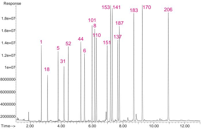
Figure 2. Chromatogram of PCB congener mixture, M-8082 from AccuStandard, 100 pg/µL in hexane.
