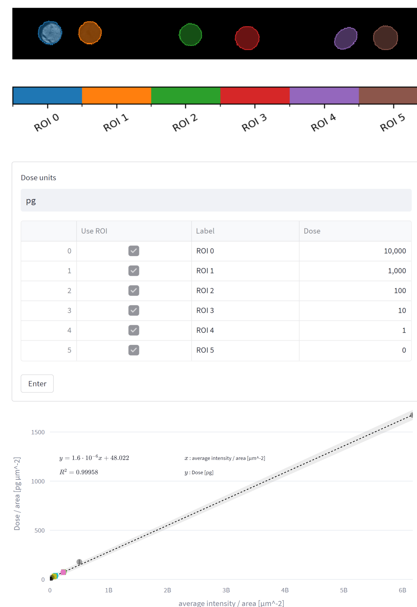
Figure 3. (Top) Visualization of regions of interest from dilution series. (Middle) Input form for custom labels, dose quantities, and units. (Bottom) Resulting calibration curve with associated confidence interval.
