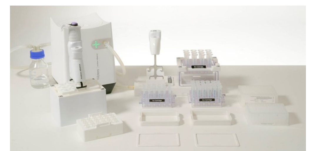
Figure 2. The Extraction+ system including the connected vacuum pump, flow-through waste container, Extraction+ manifold with the manifold collar, the integrated collar lifter, and SPE cartridges (1, 3 and 6 cc) with the corresponding adaptors.
